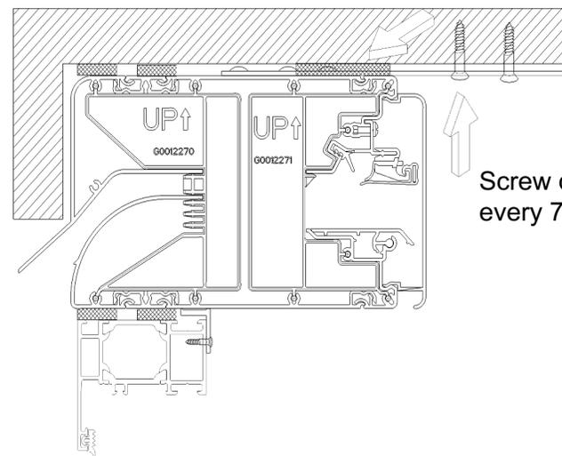
4a) Shimming window ventilator every 700 mm
