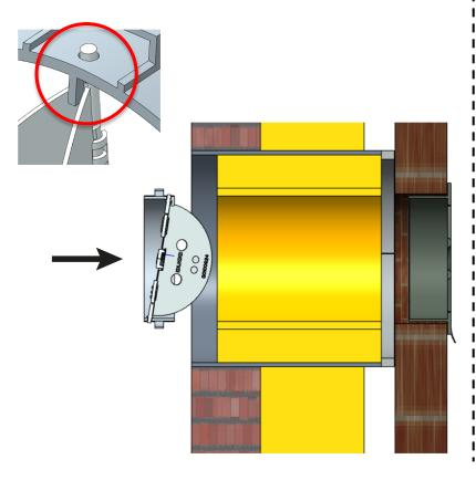
2. Apply silicone to the joint between the PVC tube and the wall for a good seal.
