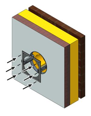
4. Slide the trim plate with the previously fitted plastic parts and sections over the sleeve bearings.
