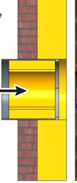
4. Slide the decorative grille into the 150 mm dia. opening. This step may also take place last. Joint sealant tape or sealant can be applied around the grille if it is not adequately secure.
