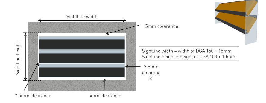
The Duco Acoustic Module 150 is available in a range of dimensions:
