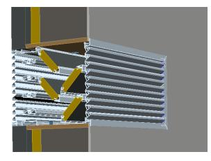
For improved acoustic performance and where the fitting depth so permits, 2 identical DAM 150 assemblies can be fitted next to one another. When doing so, turn one assembly upside down, with the result that clearance alternates between the top and bottom.
