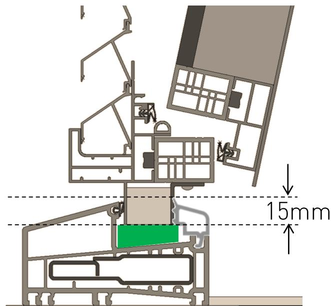
Be very careful when placing the support blocks. These should be wider than the thickness of the glass so that the DGNV is worn across the full width.
