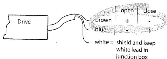
If drive operates in wrong direction interchange the connection leads to the 24V DC control power.
