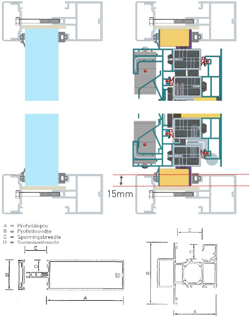
(Just like glass,) DucoGrille NightVent is mounted in the rebate of the window or façade profile - principle of sealing profiles (dry glazing).
