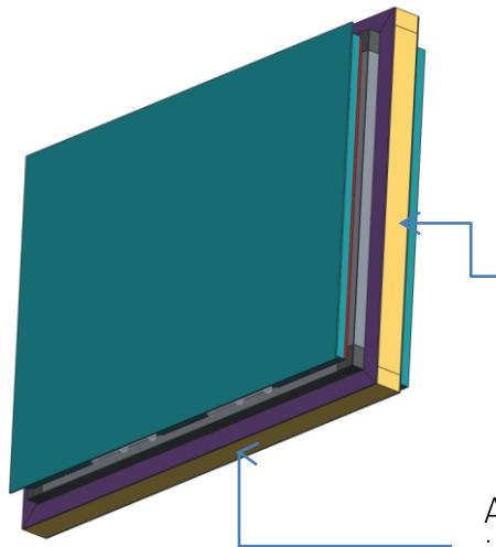
At the side and top, ensure that the support blocks are never spaced over 500mm. With small shutters there is a minimum of 2 support blocks per side.
