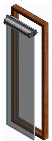
1. After it has been set in the frame, screw the window ventilator into the rebate with a countersunk sheet metal screw  $3.5 \text{ mm} \times 50 \text{ mm}$ .
