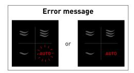
In either case, go to the DucoBox to find out exactly what message shows (DisplayMenu:  $INFO \rightarrow ERROR\ LIST$ ) and communicate this code to your installer.
