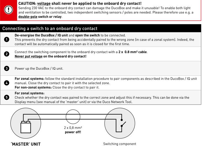
Onboard switch sensor
