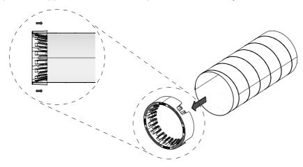
• Step 2: Clamp the duct flange together with the duct over a spigot  $\varnothing$  125 of a DucoBox until the ring touches the casing.
