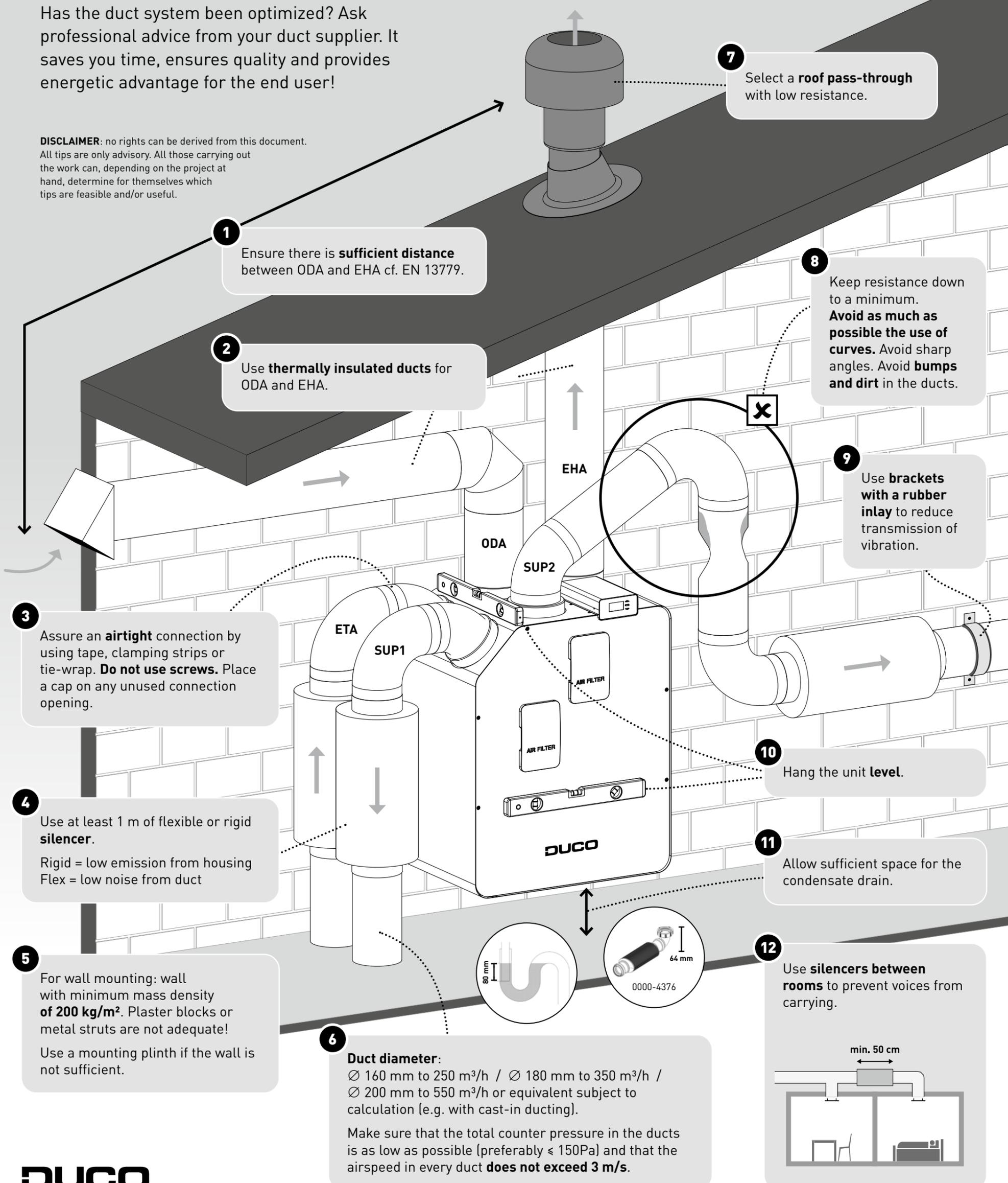
**1** Ensure there is **sufficient distance** between ODA and EHA cf. EN 13779.
